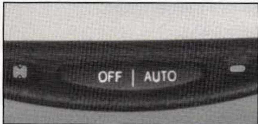
Press the OFF AUTO button at the base of the mirror to turn on the automatic feature. The button has an indicator light to show it is on. Press the OFF AUTO button to turn the automatic feature off.
