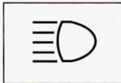
When the high beams are on, this indicator light on the instrument panel will also be on.
