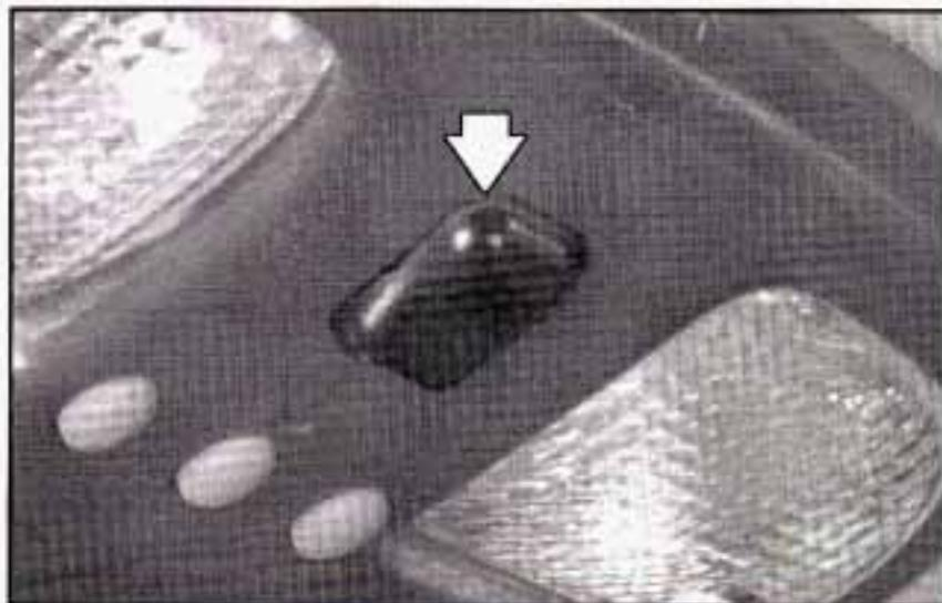
Your vehicle may be equipped with a power sliding sunroof. To open or close your sunroof, the ignition or RAP needs to be on. See “Retained Accessory Power” in the Index.
