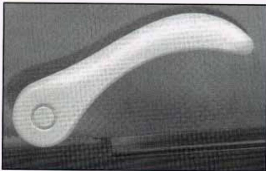
To adjust the right front passenger's seatback, lift the lever on the outer side of the seat.
