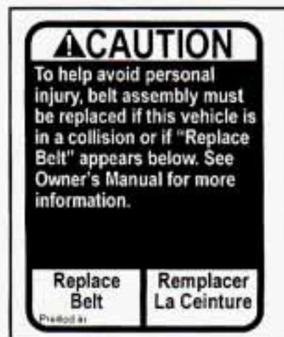
If you ever see a label on the driver's or the right front passenger's safety belt that says to replace the belt, be sure to do so. Then the new belt will be there to help protect you in a collision. You would see this label on the belt near the door opening.
