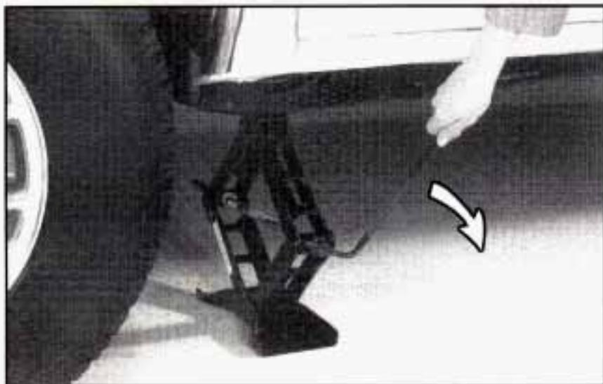
4. Raise the vehicle by turning the jack handle to the right. Raise the vehicle far enough off the ground so there is enough room for the spare tire to fit.
