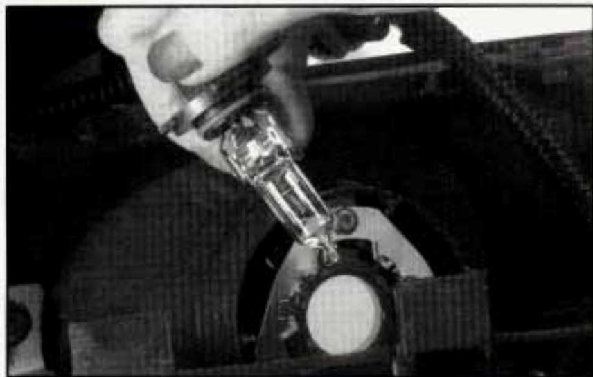
5. Turn the bulb assembly to the left to remove it.
